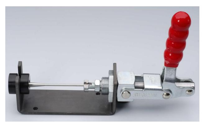
Step 1: Push tapered spindle (G) through housing until the end is nearly flush with housing.
