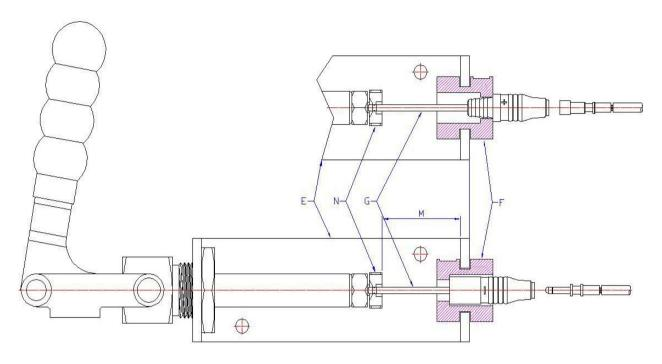
Step 4: Make sure the housing is completely assembled with the socket or pin, if it has been assembled correctly; they will be flush with the end of the housing.
